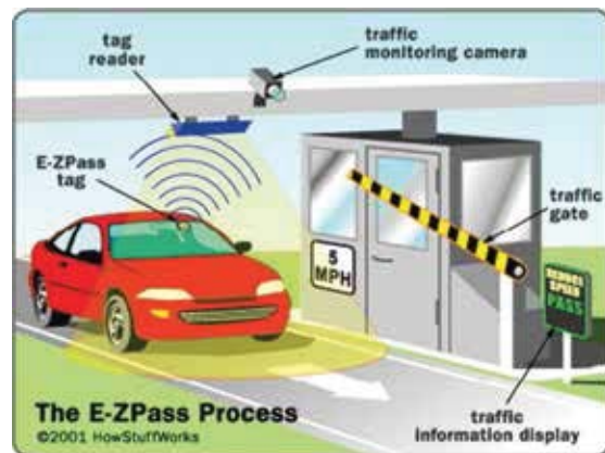
Fig. 7.5: Electronic Toll Plaza
