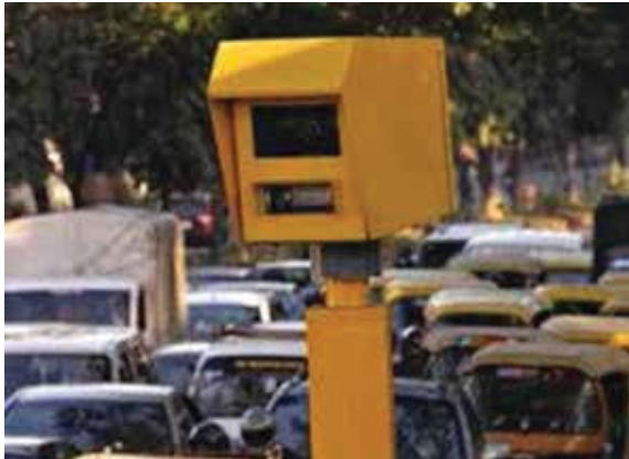
Fig. 17.4: Traffic Enforcement Camera
